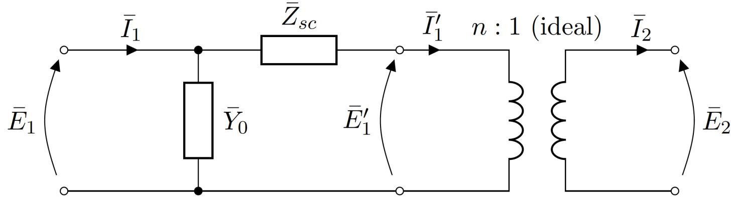
The equivalent circuit of a transformer in absolute units looks as shown above, where  $\bar{Z}_{sc}$  is the **short-circuit impedance**,  $\bar{Y}_0$  is the **zero-load admittance**, and  $n$  is the **transformation ratio**.
